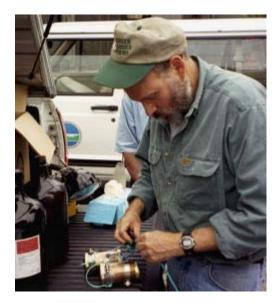
Figure 5. Preparing PISCES in the field. PISCES are usually deployed in pairs in case one fails. The bottles in the truck hold hexane.
