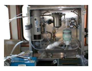
Figure 3. TOPS on the EPA' s New York Harbor Survey Vessel *Clean Waters*. The "U" shaped device near the top holds a cartridge filter and the two white double-ended cartridges hold XAD. The two small boxes in the upper right side are flow meters.
