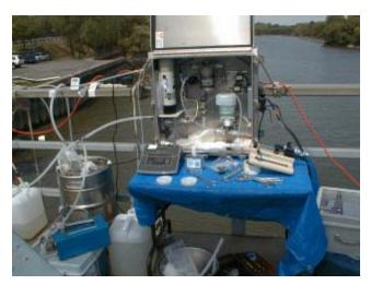
Figure 9. TOPS running on the Passaic River. Notice the stainless steel can on the left where large zooplankton are removed by filteration. A syringe pump delivering metered surrogates is seen on the table to the right of the TOPS. The plastic carboys on the deck collected water during timed intervals as an independent check of pumping rates. Note the lack of simplicity.
