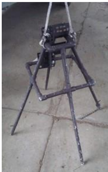
Figure 1. Frame used to mount down-looking camera for round goby video surveys.
