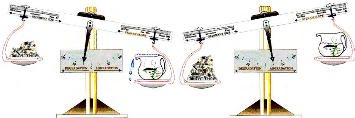
Figure 2.5a If the supply of sediment decreases or the supply of water increases, the stream will begin to erode the stream bed or degrade. (After Rosgen, 1996)
