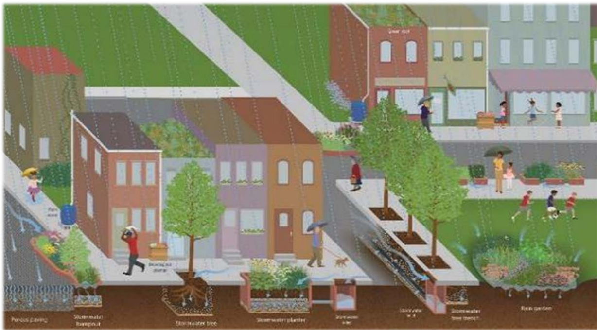
Figure 3-4. Examples of constructed stormwater green infrastructure including from left to right, porous paving, stormwater bumpout, stormwater tree, stormwater planter, stormwater inlets, stormwater tree trench and rain garden.
