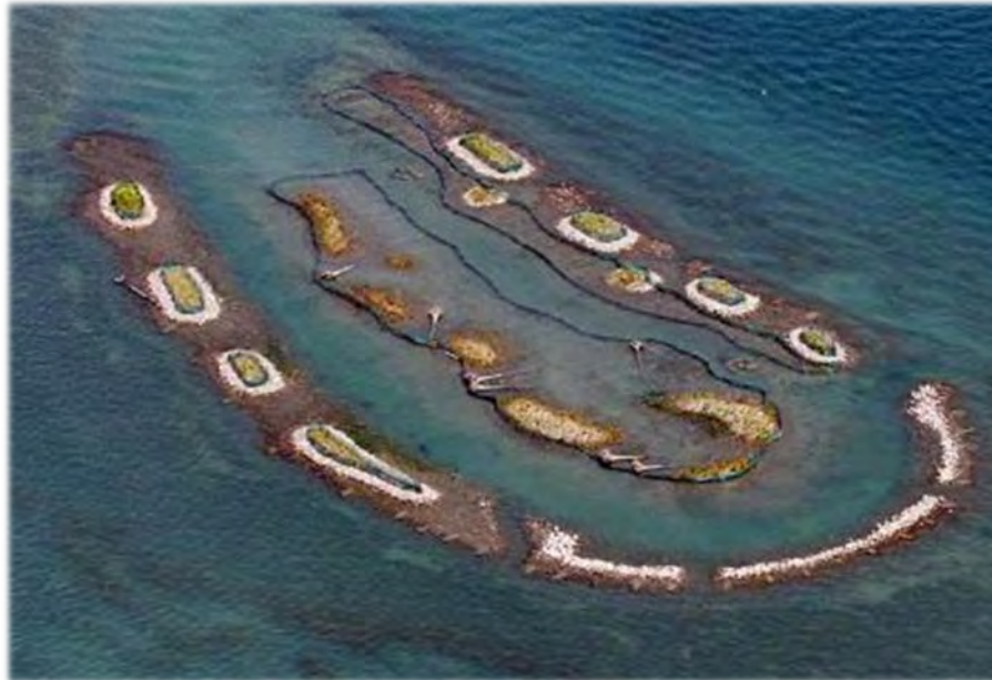
Figure A.14-5. Use of wetland sills to capture sediment and support wetland development and habitat improvement in the Niagara River.
